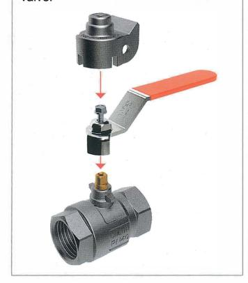
**3.** Place and lock the locking device either on the open or on the shut-off valve.
