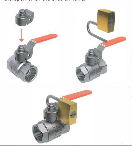
4. Place and lock the locking device either on the open or on the shut-off valve.
